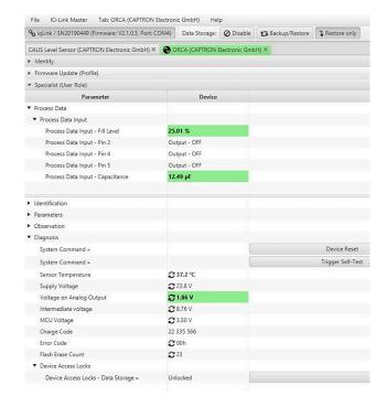
The "Reset device" system command is used to perform a warm start of the sensor. Unlike the "Set factory settings" system command, the parameterization and calibration values are retained in the device
