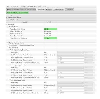
The switching point (fill level in %) and the hysteresis (difference below the switching point in %) as well as the minimum pulse time of the output can be defined and transferred.
